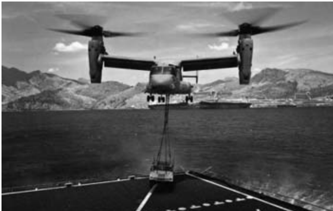
Landing support specialists back away after connecting a Humvee to a Marine Corps MV-22B Osprey during external lift training at Subic Bay, Philippines, during exercise Freedom Banner 2013. (Pfc. Kasey Peacock/Marine Corps)
